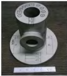
8" \text{\O} x 2" bore x 4" OD x 1/2" thick (203mm \text{\O} x 51mm bore x 102mm OD x 13mm thick)
