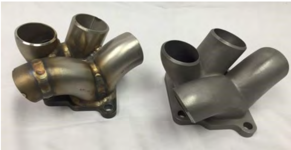
Figure 1 – An example of how additive manufacturing can eliminate weld locations in a pipe manifold [F.1].
