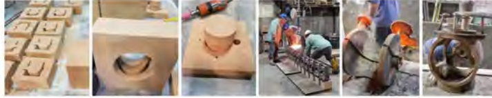
Binder Jetted Sand Casting Molds
