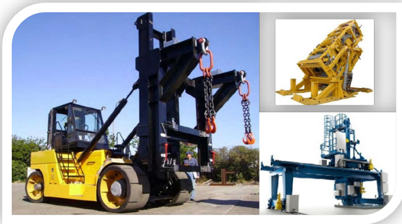
The Fuel Retrieval and Packaging System was an integrated system of remote handling equipment that enabled the harvesting of fuel from an outdoor tile array, drying of the fuel and repackaging it for indoor storage.
