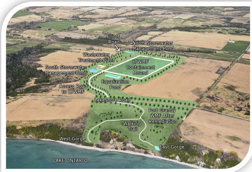
Providing value was an essential part of winning the local communities support for the remediation plan. The mound was shaped to resemble a natural landform and tilted to mimic existing drumlins in the area and walking trails will be incorporated into the remediated land.
