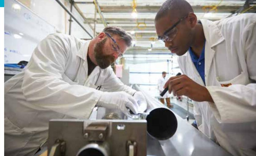
OPG workers inspect calandria tubes before installation into the Unit 2 reactor, Darlington Energy Complex.
